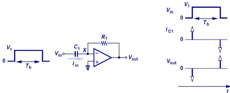
$$V_{out} = \mp R_1 C_1 V_1 \delta(t)$$
