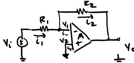
**Virtual short circuit:** Due to infinite gain of op amp, the circuit forces  $V_2$  to be close to  $V_1$ , thus creating a virtual short.
