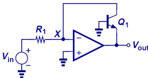
$$V_{out} = -V_T \ln \frac{V_{in}}{R_1 I_S}$$
