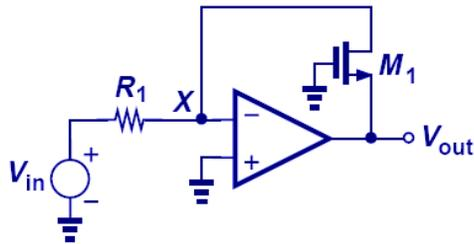
$$V_{out} = - \sqrt{\frac{2V_{in}}{\mu_n C_{ox} \frac{W}{L} R_1}} - V_{TH}$$
