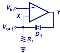
Insert a diode to "break" connection and hold X at zero during negative cycles. Assume  $V_{in}=0$ ; the opamp raises  $V_y$  to  $V_{D,on}1$  to hold X at roughly zero. If  $V_{in}$  becomes positive, X tracks. If  $V_{in}$  becomes negative,  $V_y$  goes negative. Since D1 cannot carry current (reversed biased), the opamp produces a very large negative output (near the negative rail).
