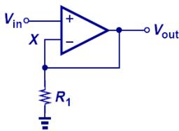
Assume a unity-gain buffer tied to the resistive load. High gain of opamp ensures X tracks  $V_{in}$ .
