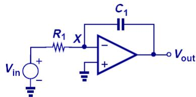
$$\omega_{int} = \frac{1}{R_1 C_1} \quad \text{Is the integrator frequency}$$
