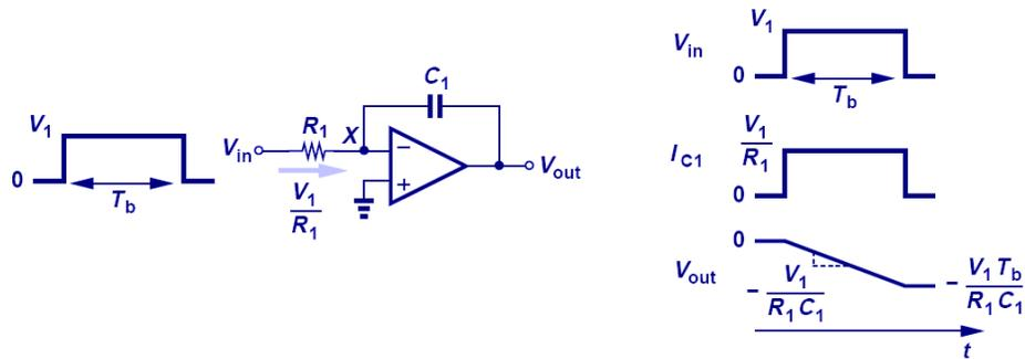
$$V_{out} = -\frac{1}{R_1 C_1} \int V_{in} dt = -\frac{V_1}{R_1 C_1} t \quad 0 < t < T_b$$
